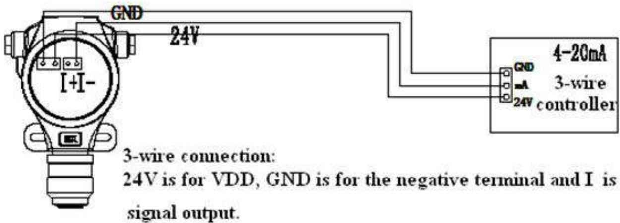
**The connection of the detector and external device**
